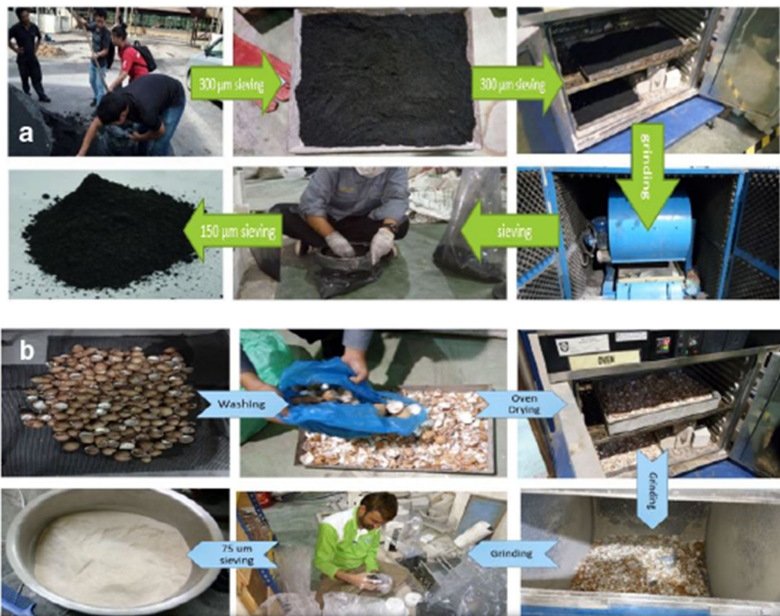
Fig. 4 Preparation process of a POFA and b ESP
