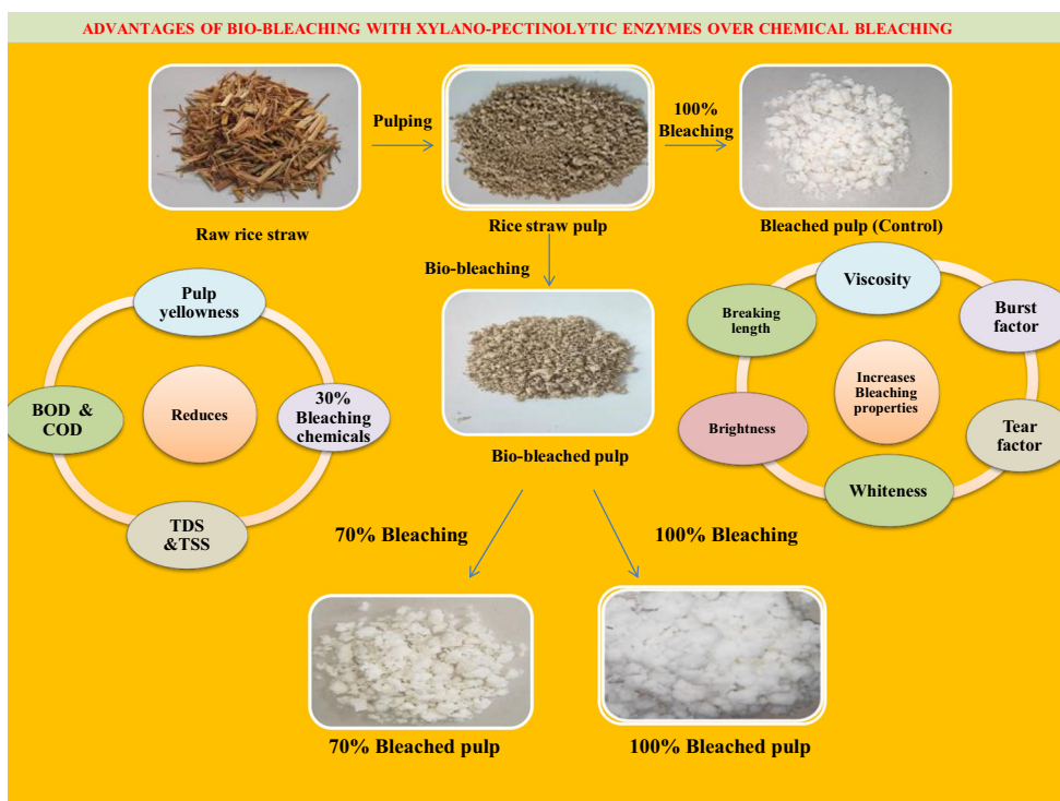
Fig. 4 Experimental summary of bio-bleaching process for rice straw pulp
