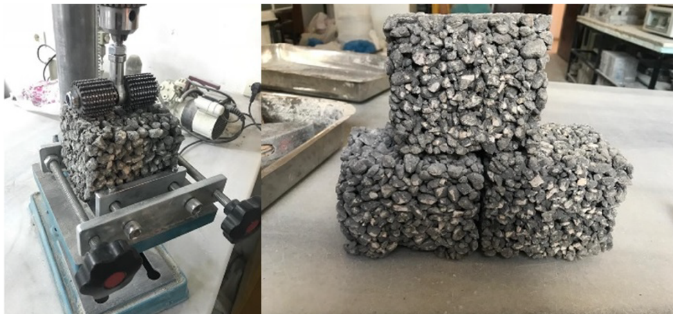
Fig. 5 Pervious concrete sample for the abrasion test according to ASTM C 944
