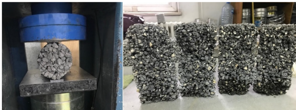
Fig. 4 Pervious concrete samples for the splitting tensile strength test
