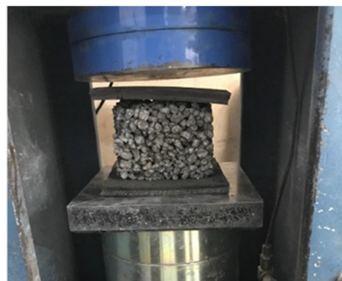
Fig. 3 Compressive strength test applied to pervious concretes
