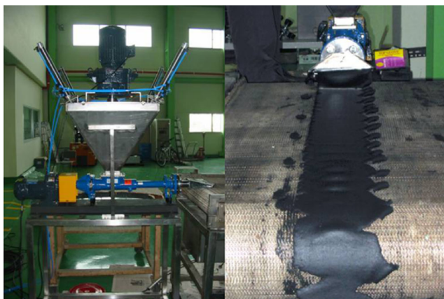
Fig. 7 The picture of nozzle-type sludge sterilisation system. Image courtesy of Kim et al. (2009)
