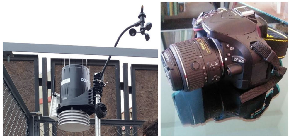
Fig. 3 Meteorological station Davis Vantage Pro 2 and fisheye lens + Nikon Camera D5200
