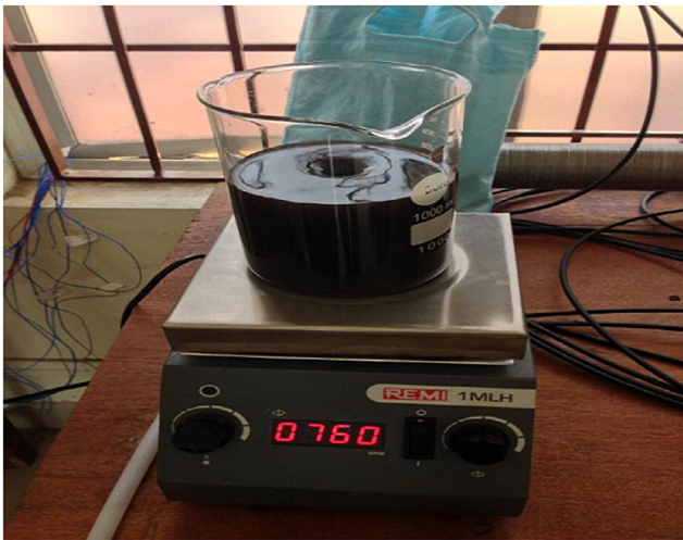
Fig. 9 Magnetic stirrer to ensure uniform dispersion for CuO nanofluid
