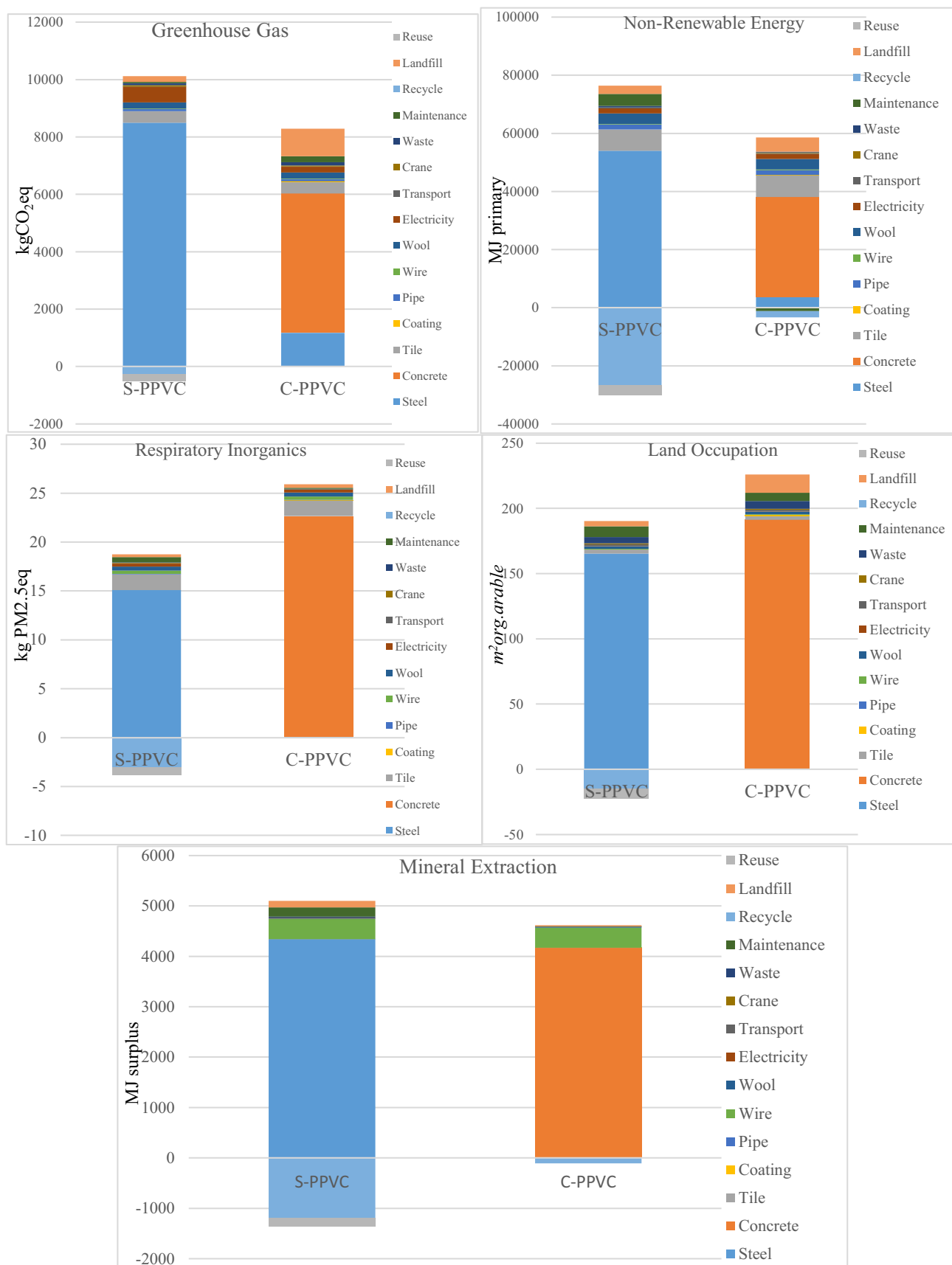
Fig. 6 Detailed comparison of the two PPVC structures (i.e., steel (S-PPVC) and concrete (C-PPVC))
