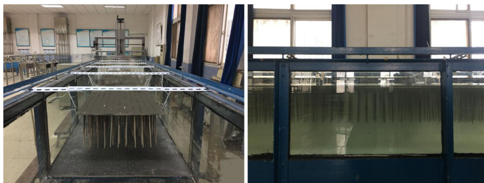
Fig. 2 Experimental setup showing the placement of FVIs in the flume
