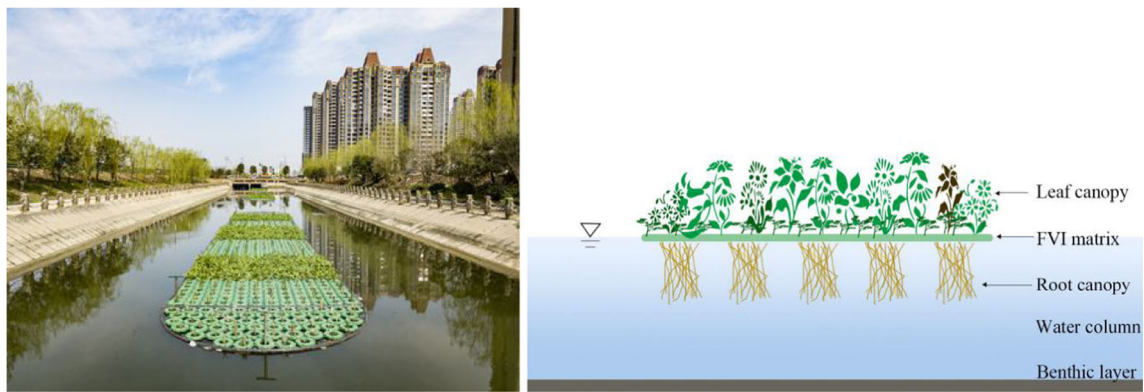
Fig. 1 Photo and schematic of FVI system
