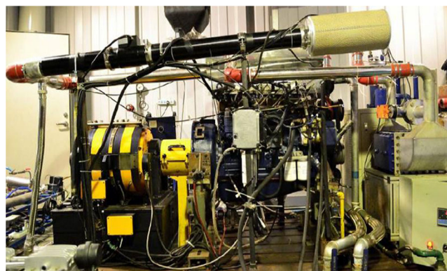
Fig. 3 A six-cylinder turbocharged common rail DME engine
