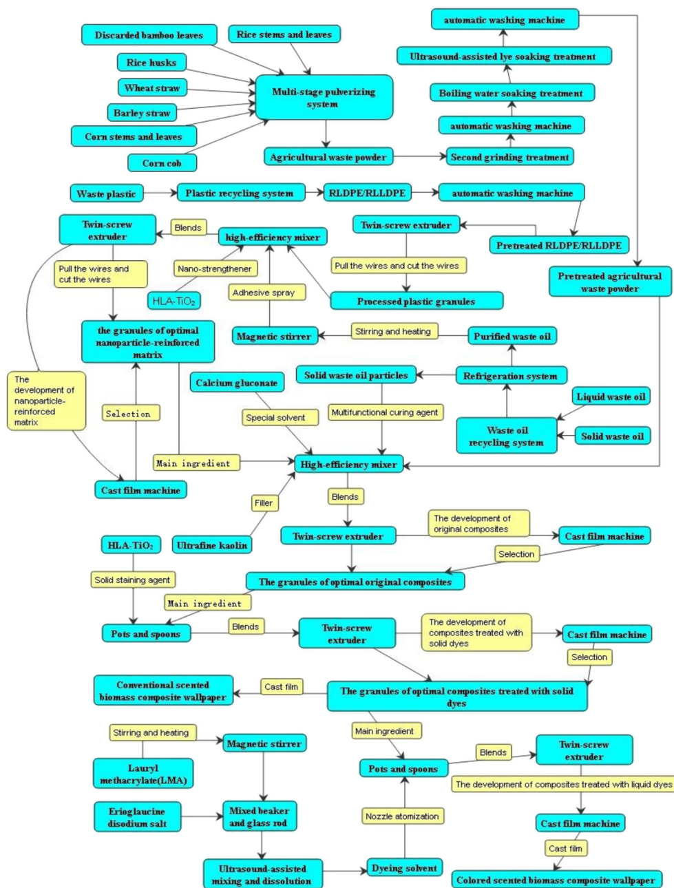
Fig. 4 The processing system of the development of high value-added new biomass composite wallpaper
