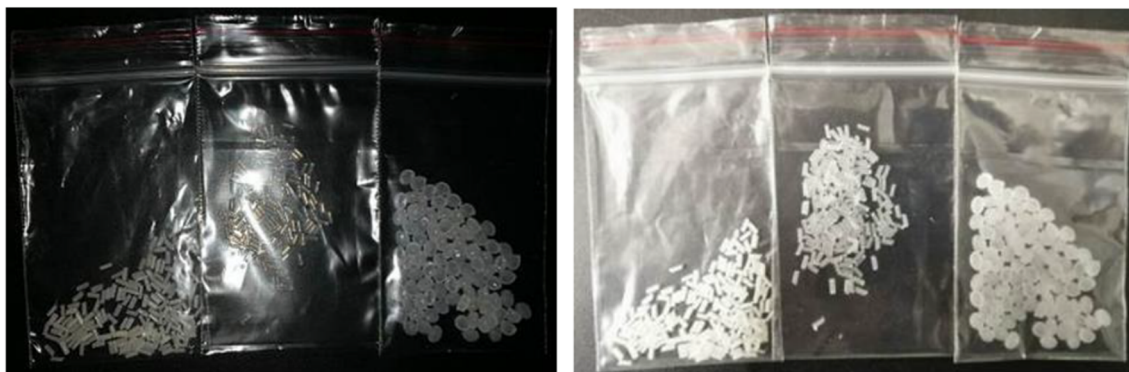
Fig. 6 Physical photos small cylindrical RLDPE granules, small cylindrical granules no. 1, and ellipsoidal normal plastic granules
