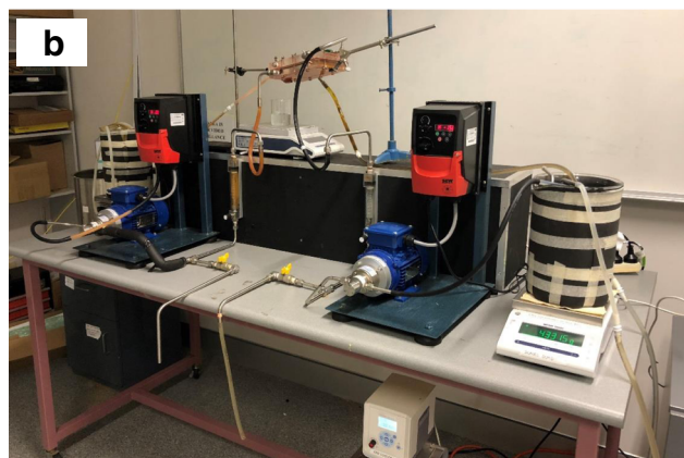
Fig. 1 a A schematic diagram and b a real picture of the lab-scale MD system
