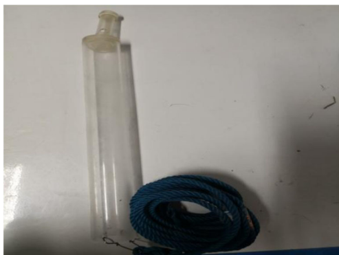
Fig. 5 Underground water sample collector
