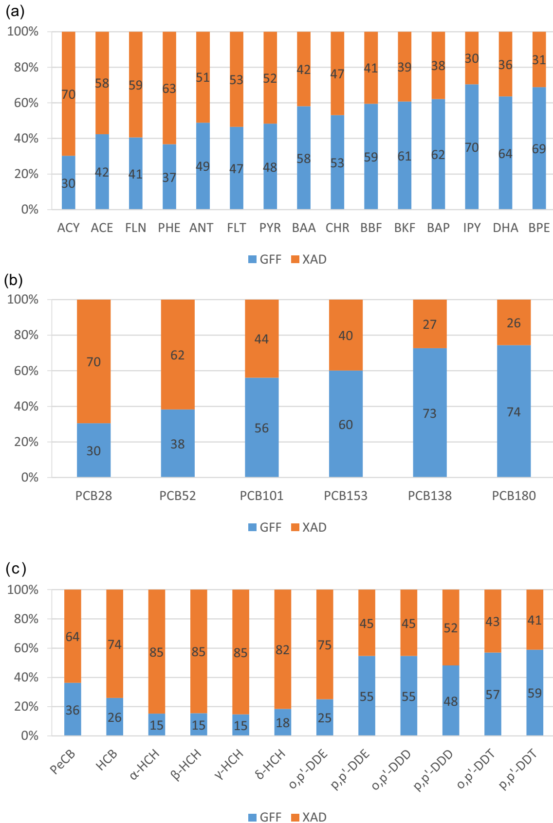
Fig. 3 Average distribution between GFF and XAD of a PAHs, b PCBs and c OCPs
