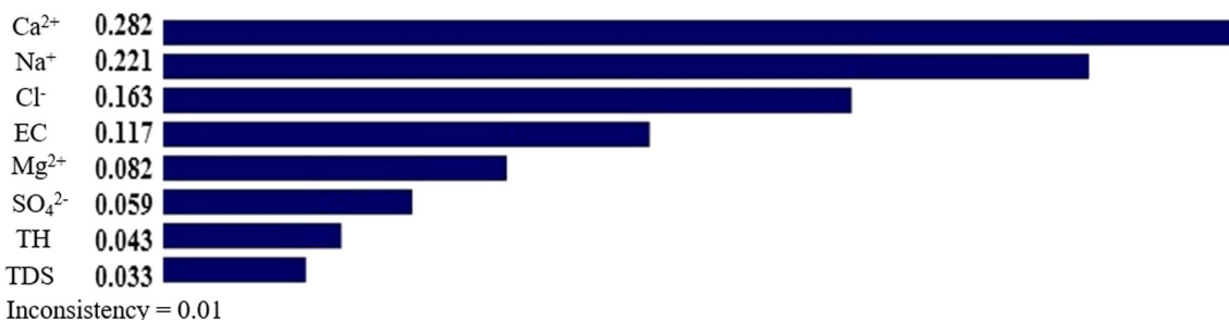
Fig. 7 Weights assigned to each water quality constituent for creating the overall water quality index in the fuzzy AHP model
