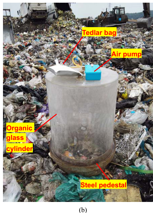
Fig. 3 Static chamber used for monitoring of landfill gas: (a) schematic of static chamber (mm); (b) static chamber on the working face
