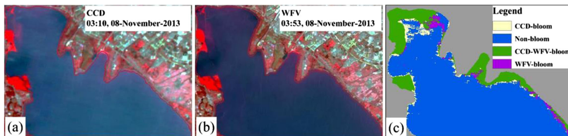
Fig. 5 Comparison of the bloom area derived from HJ-1/CCD and GF-1/WFV on 8 November 2013. a False-color composite image by WFV. b False-color composite image by CCD. c Comparison of the extracted bloom area of the two sensors. Non-bloom, non-bloom water for both
