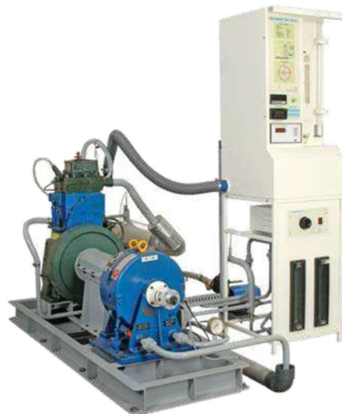
Fig. 2 Photographic view of test engine
