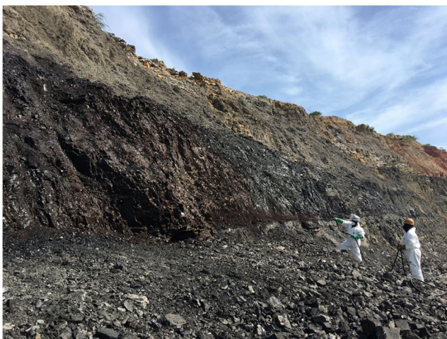
Fig. 6 Application of bitumen on the coal seam
