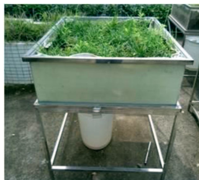
Fig. 2 Green roof profile (1 vegetation layer, 2 substrate layer, 3 filter layer, 4 storage layer, 5 perforated collector, 6 Perspex outer wall, 7 stainless steel bracket) and a picture of studied green roof
