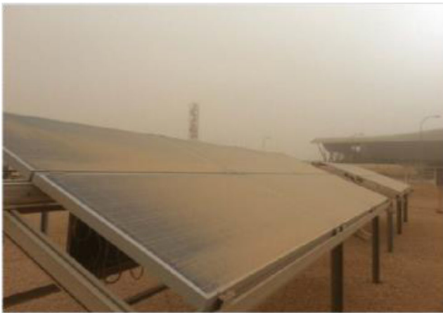
Fig. 4 Soiling of solar panels at the Solar Test Facility in Doha (The State of Qatar) after dust storm in 2014 (Aissa et al. 2016)
