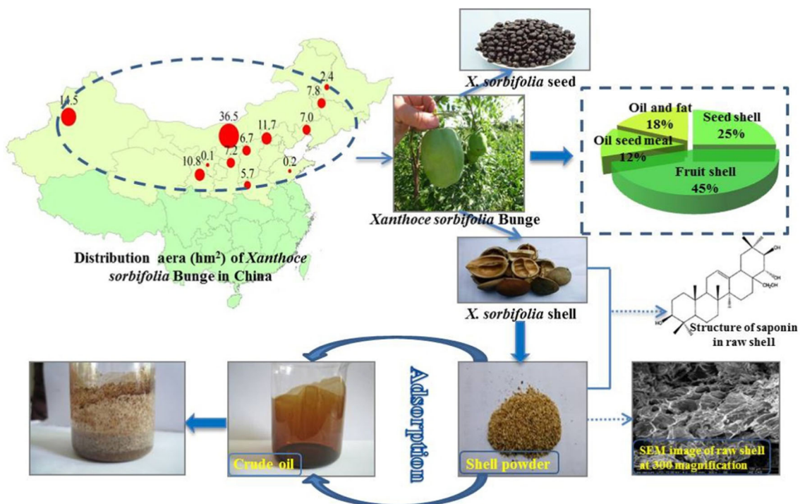
Fig. 1 Source and primary characteristics of the raw Xanthoceras sorbifolia shell and the adsorption process for crude oil
