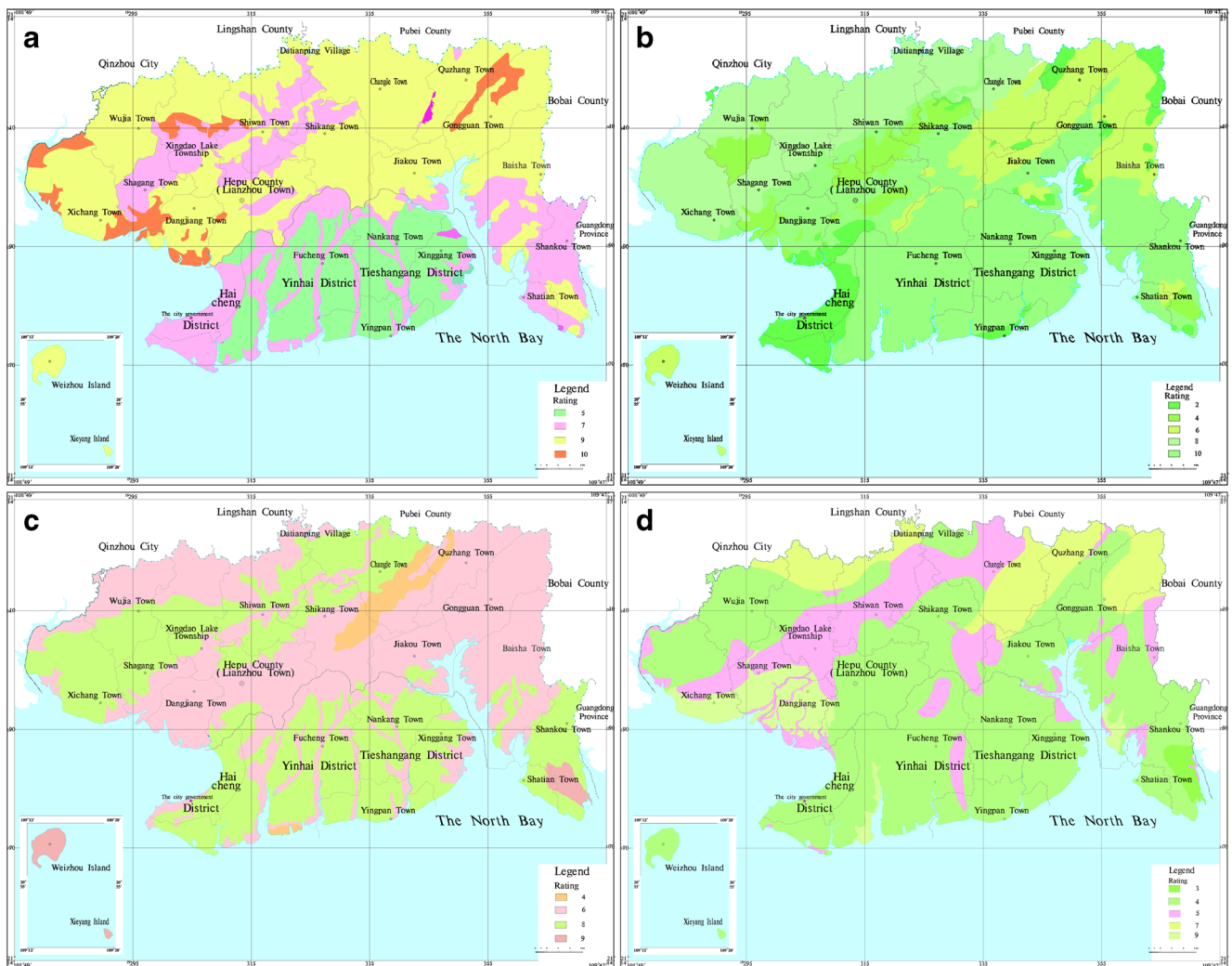
Fig. 7 Rating distribution map of groundwater vulnerability other indexes: (a) depth of groundwater table, (b) rainfall recharge, (c) aquifer media, and (d) soil media
