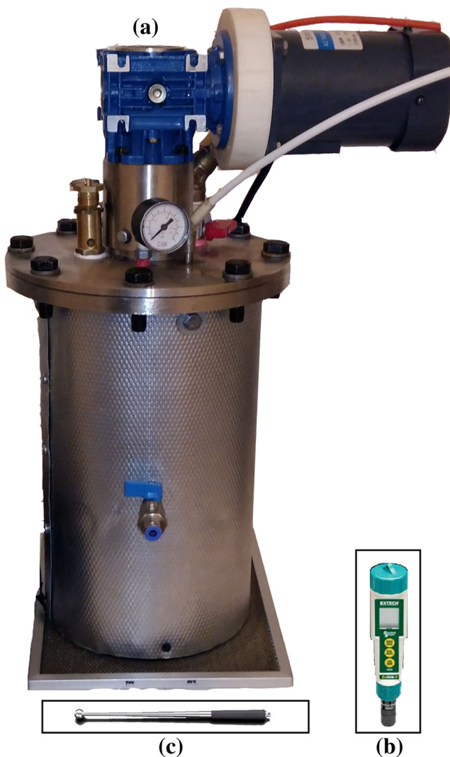
Fig. 1 Experimental set-up: lagged bioreactor (a). DO meter electrode (b). Spherical probe for electro-diffusion method (c)
