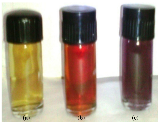
Fig. 3 Camera images of a aqueous M. glabrata leaf extract, b AgNP- M. glabrata , and c AuNP- M. glabrata
