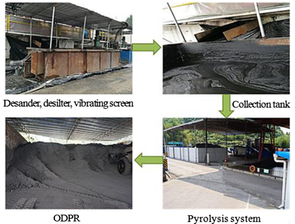
Fig. 4 Treatment processes of oil-based drillings
