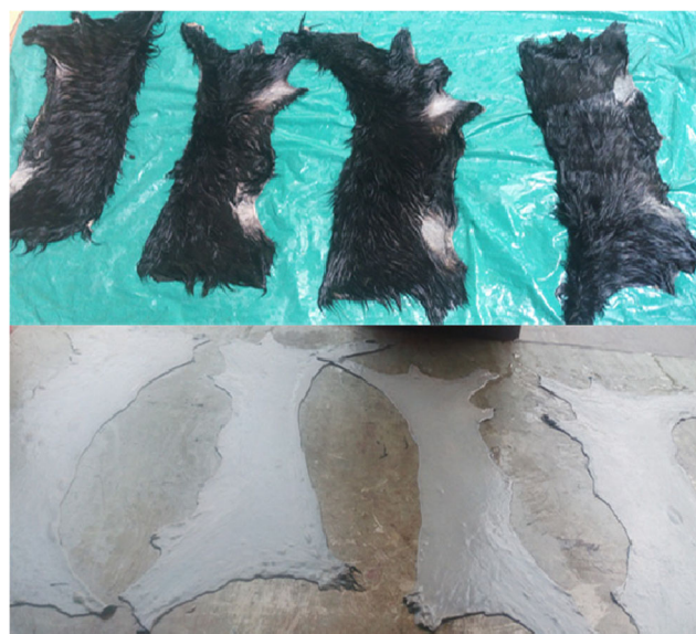
Fig. 4 Soaked goat skins (above) and drum-based SSF enzyme unhaired goat skins (below) (using fermented bran)
