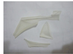
c Film formed by corn starch mixed with 30% of glycerol
