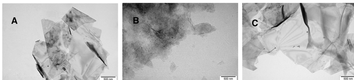
Fig. 1 TEM images of pristine graphene (a), graphene oxide (b), and reduced graphene oxide (c)
