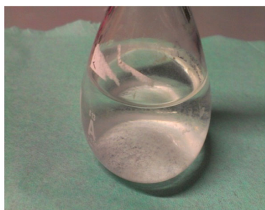
White precipitate formed in carbonated NaOH solution made in Ca solution
