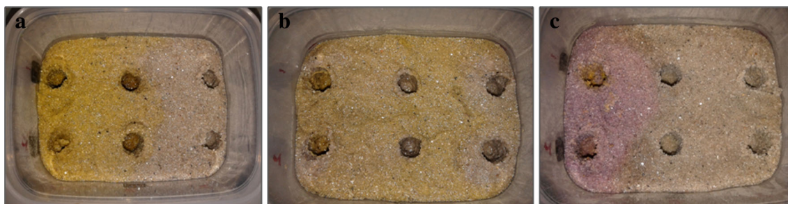
Fig. 3 Physical observation of soil after the experiments: a 0.1 M NaNO 3 , b 0.1 M citric acid, and c 0.1 M EDTA (anode region ( left section ), S1; cathode region ( right section ), S4)
