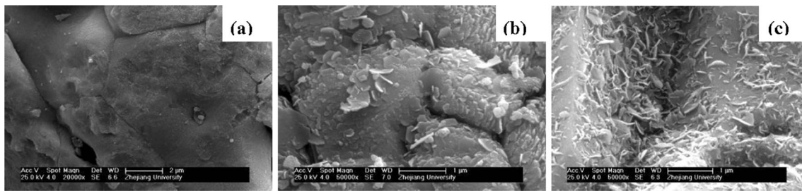
Fig. 5 SEM images of RZVI surface in different anaerobic systems: a \times 20,000 , RZVI (before reaction); b \times 50,000 , from RZVI control system (after reaction); and c from combined RZVI-anaerobic sludge system (after reaction)
