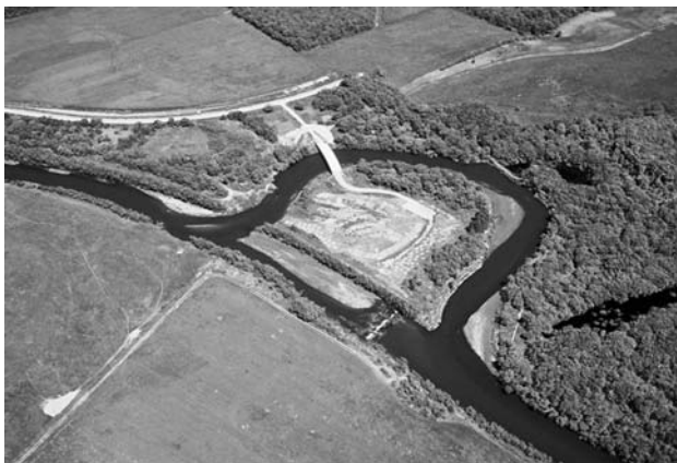
Fig. 1 Photograph of the experimental restored meandering reach in the Shibetsu River, northern Japan
