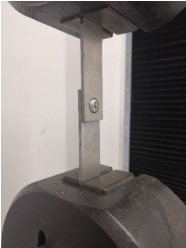
Fig. 6 Quasi-static tensile loading of the single-lap rivet-bonded hybrid joint
