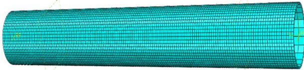
Fig. 4 Finite element model and meshing of thin-walled tube torsion test
