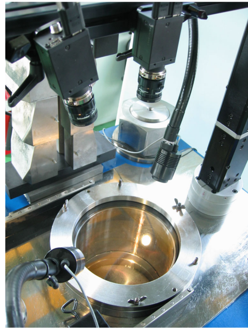
Fig. 7 View of the bulge test experimental set-up
