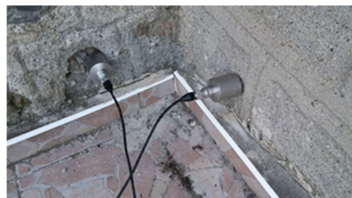
Fig. 2 The accelerometer connections
