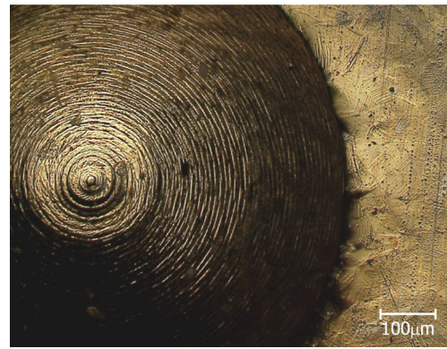
Fig. 11 A magnified image showing little pile-up around a machined lens
