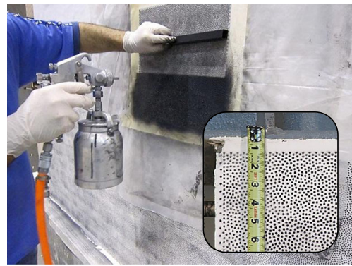
Fig. 8 Spray-painting of speckle pattern on whitewashed background using stencil. Inset shows close-up view of finished pattern
