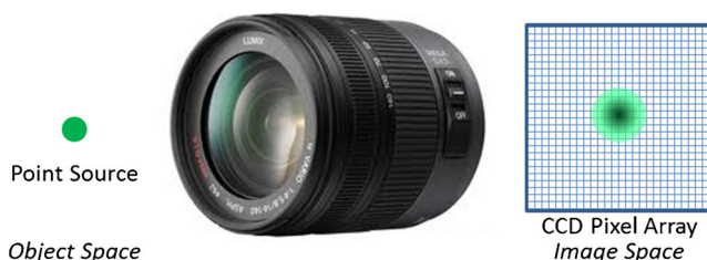
Fig. 1 Illustration of OTF and PSF for a typical lens. Illustrated is a point source in the object space and the resulting PSF on the CCD detector in the image space
