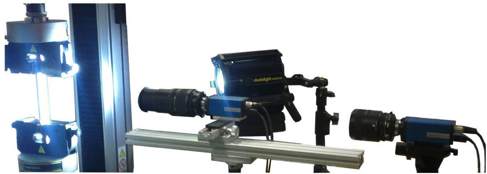
Fig. 7 Experimental setup. The two digital cameras are facing the specimen: their optical axis is perpendicular to the laminate plane. Here, a translation stage is used to retract the nearfield camera in order to capture the farfield image
