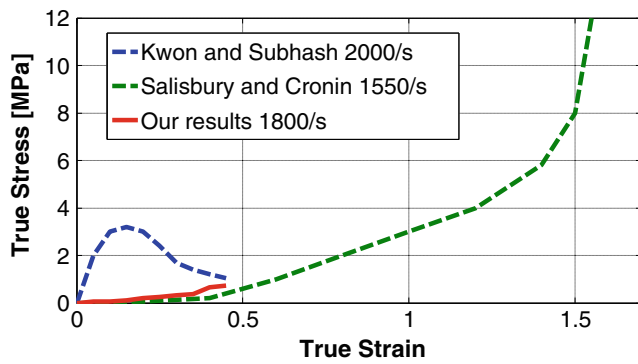
Fig. 14 BG high strain rate response as measured by 3 separate research groups for 10 % concentration
