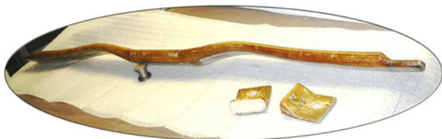
Fig. 28 Composite crossmember designed for implementation in a line of large automobiles. Also shown are two of the end pieces that were used to test various schemes for attaching the crossmember
