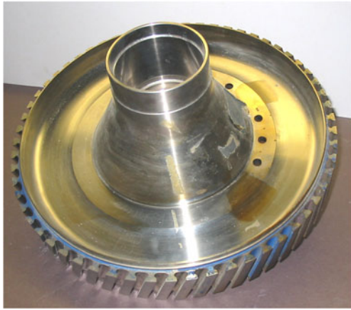
Fig. 13 Jet engine rotor used for an investigation of the effects of coldworking the mounting holes. Note the moiré gratings that were created in photoresist (the yellow coating) in the regions surrounding three of the holes
