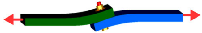
Fig. 15 Sketch of the single-lap bolted joint showing the secondary bending caused by axial load
