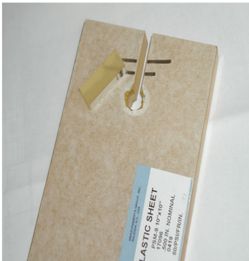
Fig. 18 Early step in the fabrication of an embedded polariscope specimen for 3-D photoelasticity analysis of the stresses in the bearing region of a bolted single-lap joint of “thick” isotropic plates
