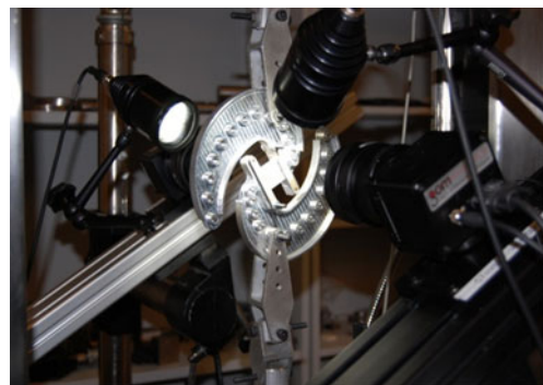
Fig. 3 2D DIC measurement set-up
