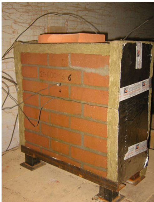
Fig. 4 Masonry specimen with applied thermocouples
