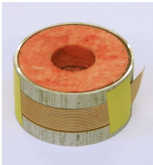
Fig. 2 A photograph of a ring sample with the make-foil gauge attached
