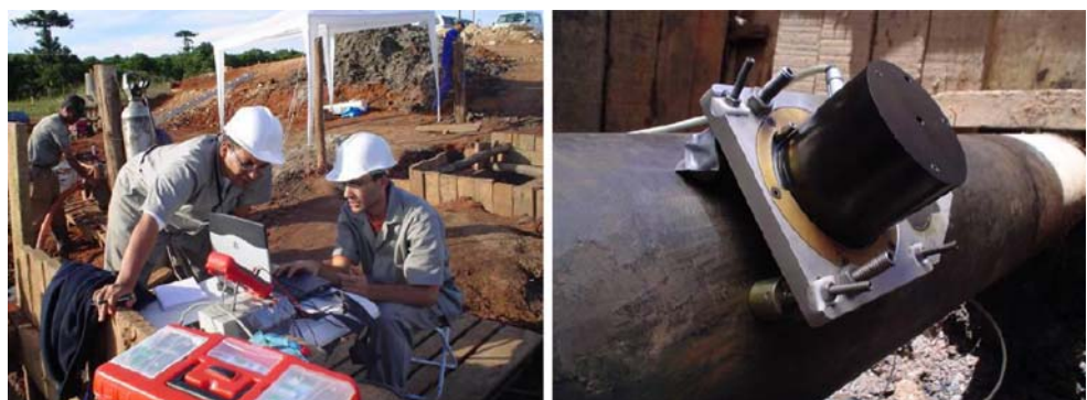
Fig. 12 Radial, in-plane speckle interferometer-hole drilling device being used to measure the stresses in a pipe induced by ground movement [89]
