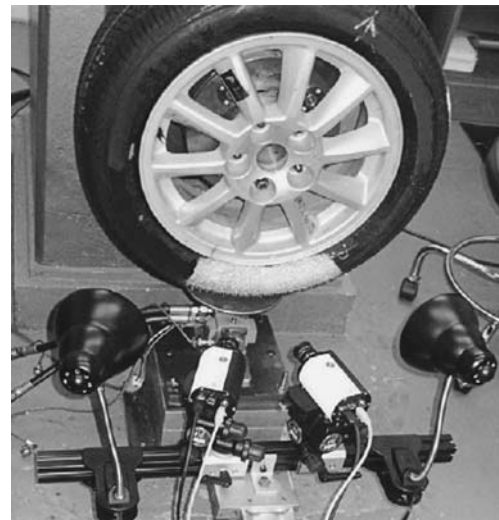
Fig. 16 Digital image correlation set-up for measurement of tire deformations showing two cameras and lamps [105]
