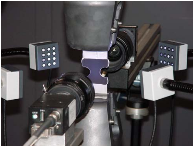
Fig. 4 Picture of the mechanical and optical set-up
