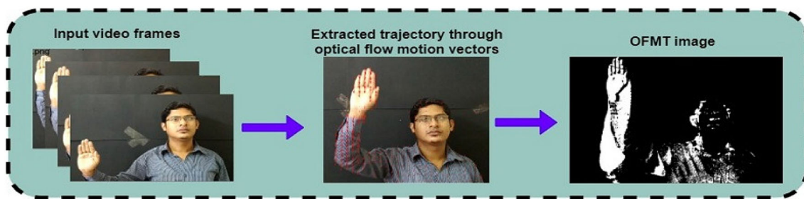
Fig. 6 Steps to obtain OFMT images from input video frames
