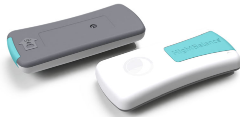
Fig. 1 The sleep position trainer (SPT). The SPT is a small, lightweight device ( 72 \times 35 \times 10 mm; 25 g) that is worn across the chest using a neoprene torso strap
