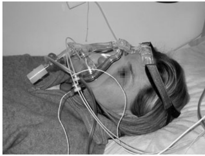
Fig. 1 Facial mask used to measure breathing variables and allowing mandibular forces on the oral appliance to be recorded
